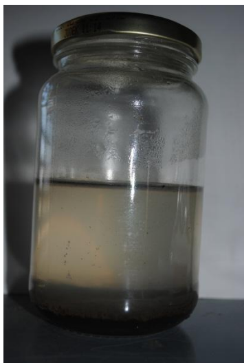
Fig 1 Oakey roof wash 0.6km from railway (settled). Photo NL
